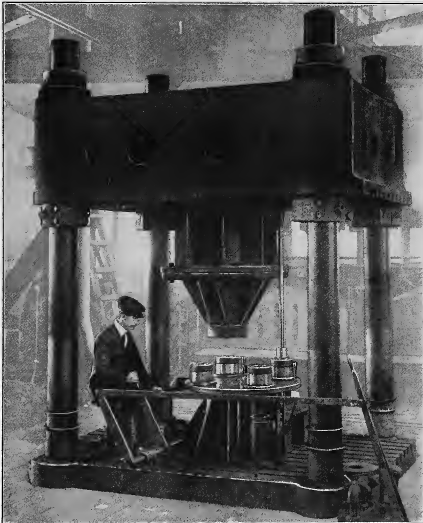
FIG. 1. A STATION-TYPE INDENTING PRESS BUILT AT ANGUS
